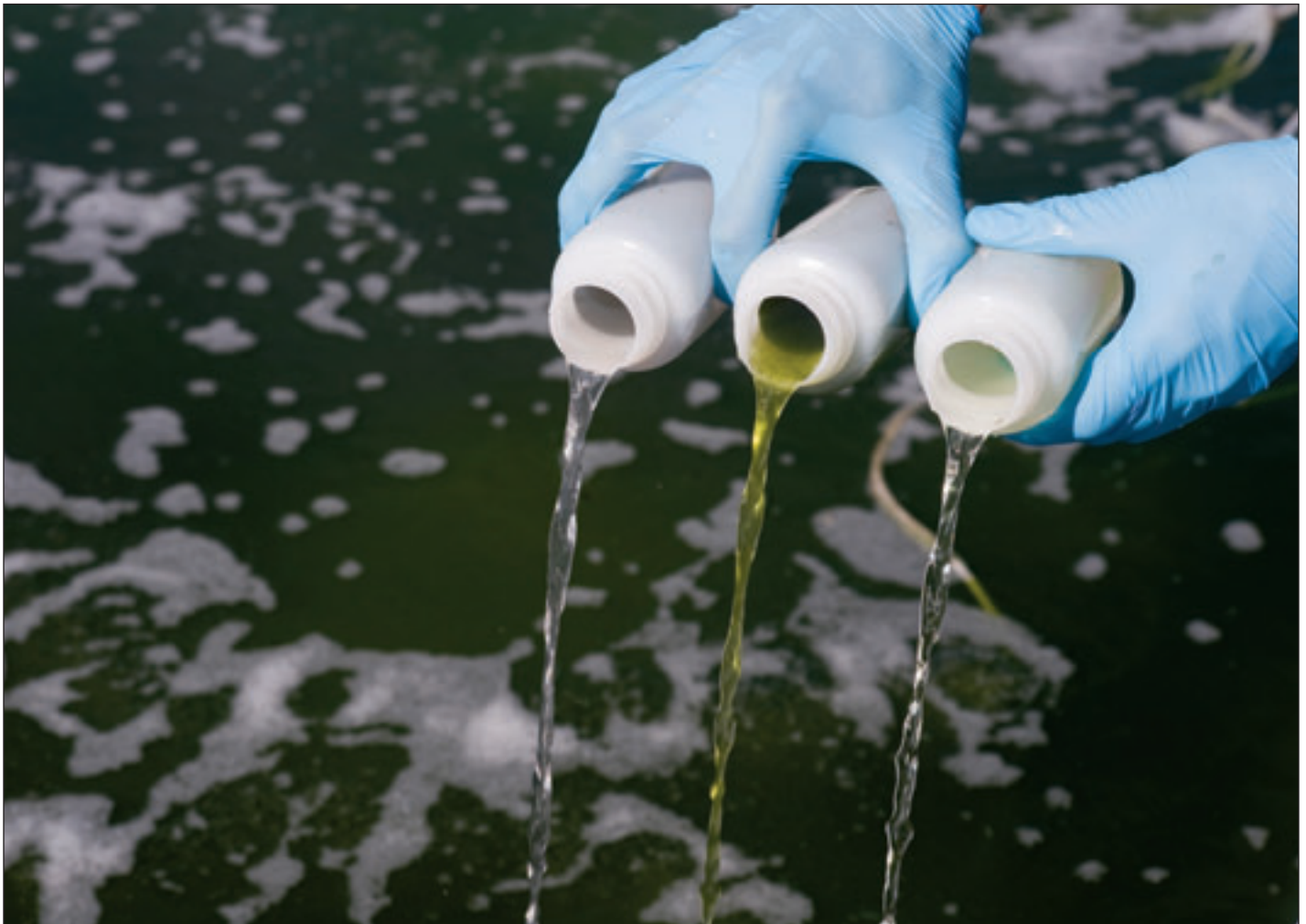
Algae consume nutrients in wastewater. Murky wastewater pouring from the bottle at the left turns green when algae is added, as in the center stream. The result is crystal clear wastewater after the algae treatment, as shown on the right. (Photo by A. Sue Weisler)
