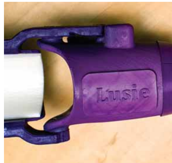
3 The students 3D-printed a custom nameplate and attached it to the arm with adhesive. Lusie had asked the students to make the arm purple but the nameplate was a surprise.
