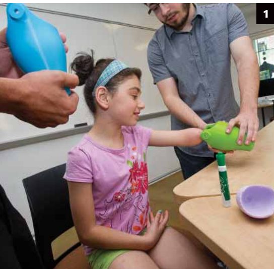
1 The RIT team had to create several versions of Lusie Santangelo’s arm in order to make it the lightest weight possible. This summer, she tried on a forearm cup from the first design that made the arm too heavy.
