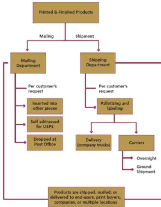
Figure 5. Distribution workflow for a mid-sized commercial printer with fulfillment center click to view full size
