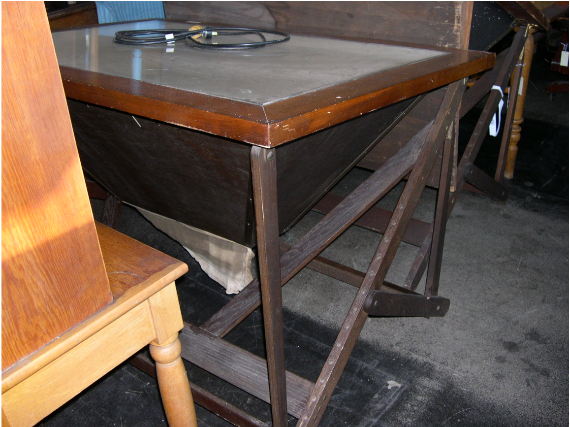
Figure 3.18: Calumet and Hecla Light Table. Note adjustable legs and trapezoidal body shape. Item 82756, Accession KEWE-00040, Keweenaw National Historical Park, Calumet, MI. Photo by Eric Nystrom, 2006.
