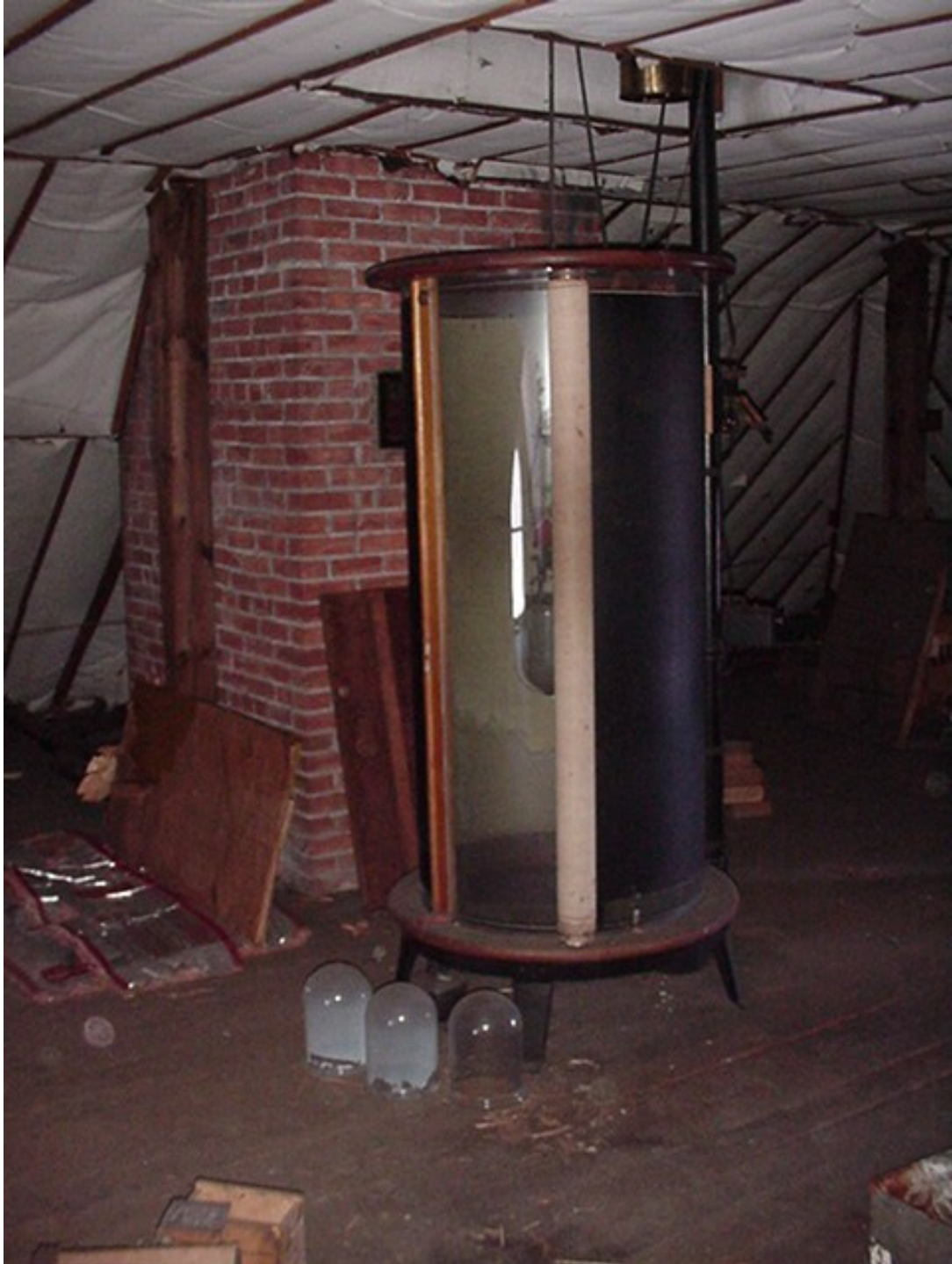
Figure 3.4: Arc Lamp Blueprint Machine, in situ in the attic of the Quincy Mining Company office building, Keweenaw National Historical Park, Hancock, MI. Photo courtesy of the National Park Service, 2001.
