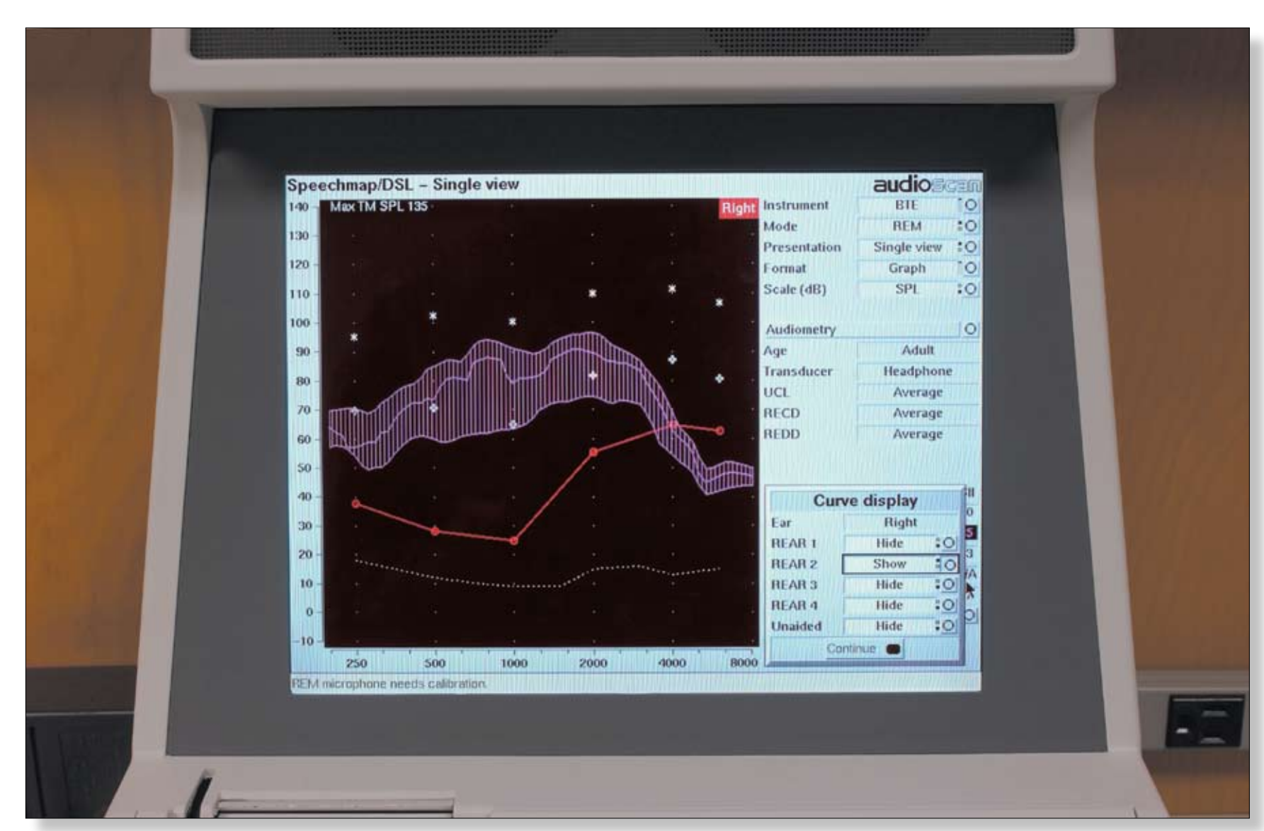
Figure 2 Measure of average speech. Purple area shows output at the ear canal. White stars show target (prescribed) fitting area.
