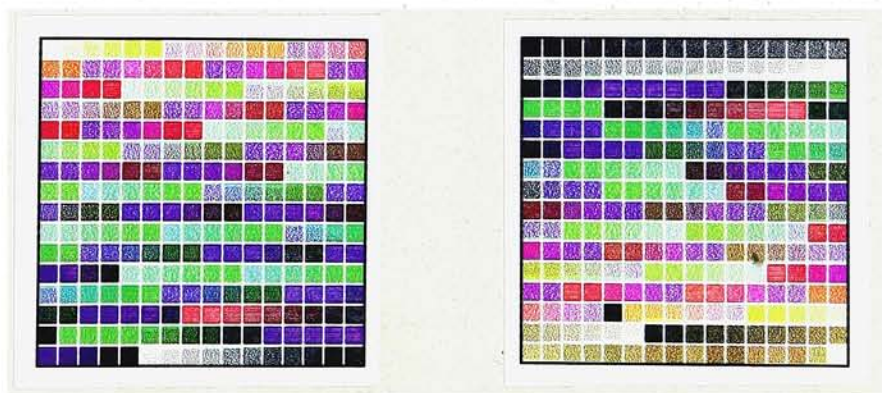
On the left hand side, the default system clut. Next to it, the custom-made clut. The main differences are a wider range of grays (at the bottom) and cream colors (at the top). The remaining colors are extracted from the system clut.
