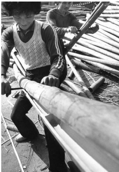
Figure 10: Traditional ways of splitting bamboo
