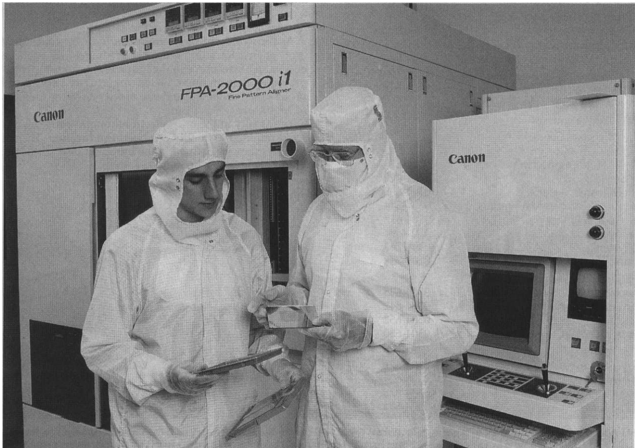
Students discuss how to use the i-line stepper to etch barely visible images on wafers in the photolithography bay.
