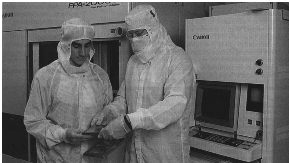
Students discuss how to use the i-line stepper to etch barely visible images on wafers in the photolithography bay.
