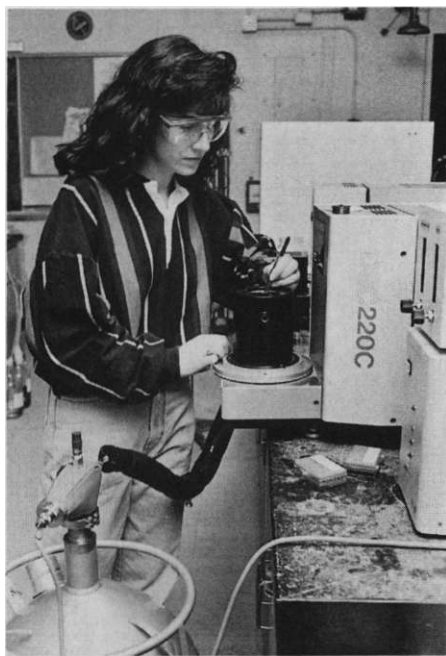
RIT's science and engineering laboratories feature up-to-date equipment and technology, such as this differential scanning calorimeter used for thermal analysis of materials.
