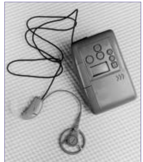
Wired for sound The external components of a cochlear implant include a microphone worn behind the ear, speech processor, and a coil placed on the skin behind the ear to send signals to the implanted components.
