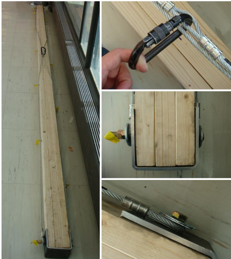
Figure 4-1 The trial beam is attached to the carabiner, the clamper, the wire, and the bolt.
