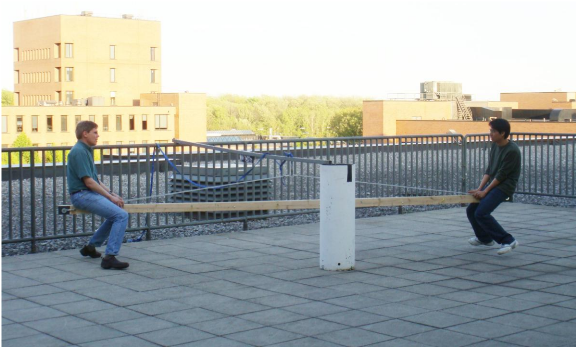
Figure 4-3 A 16-foot long wood beam is built first for simulation and tests.
