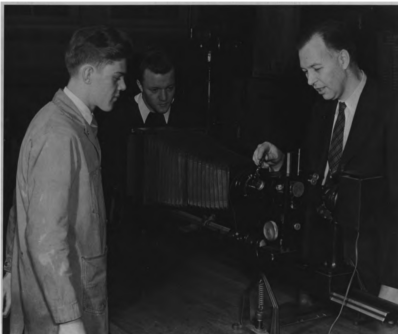
Photography has long been a part of RIT. In this recollection from an earlier decade, courtesy of the Wallace Library Archives, Instructor John Elberfeld and two of his students examine a micrograph for photographing the internal structure of metals.
