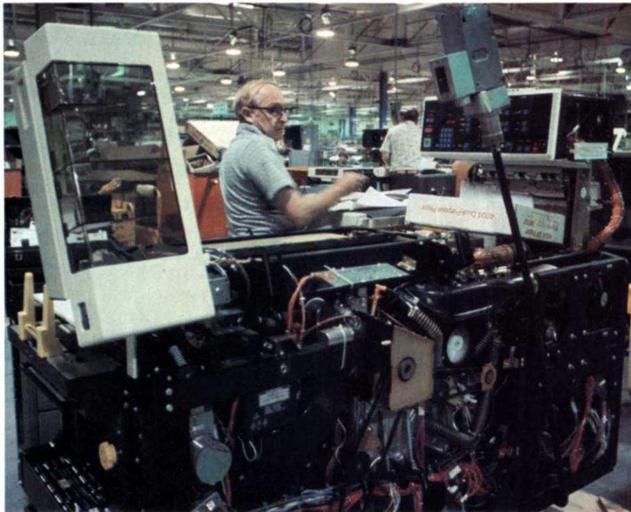
Xerox production employee assembles one of Xerox's latest products, the 9400. The 9400 can produce 7200 copies an hour, or two a second, faster than many conventional printing processes.
