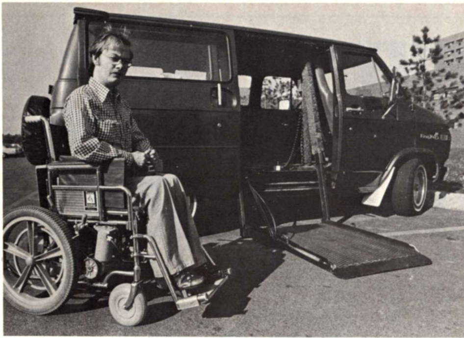
Brad Landon's van utilizes a lift but is useless if a car is parked next to it.
