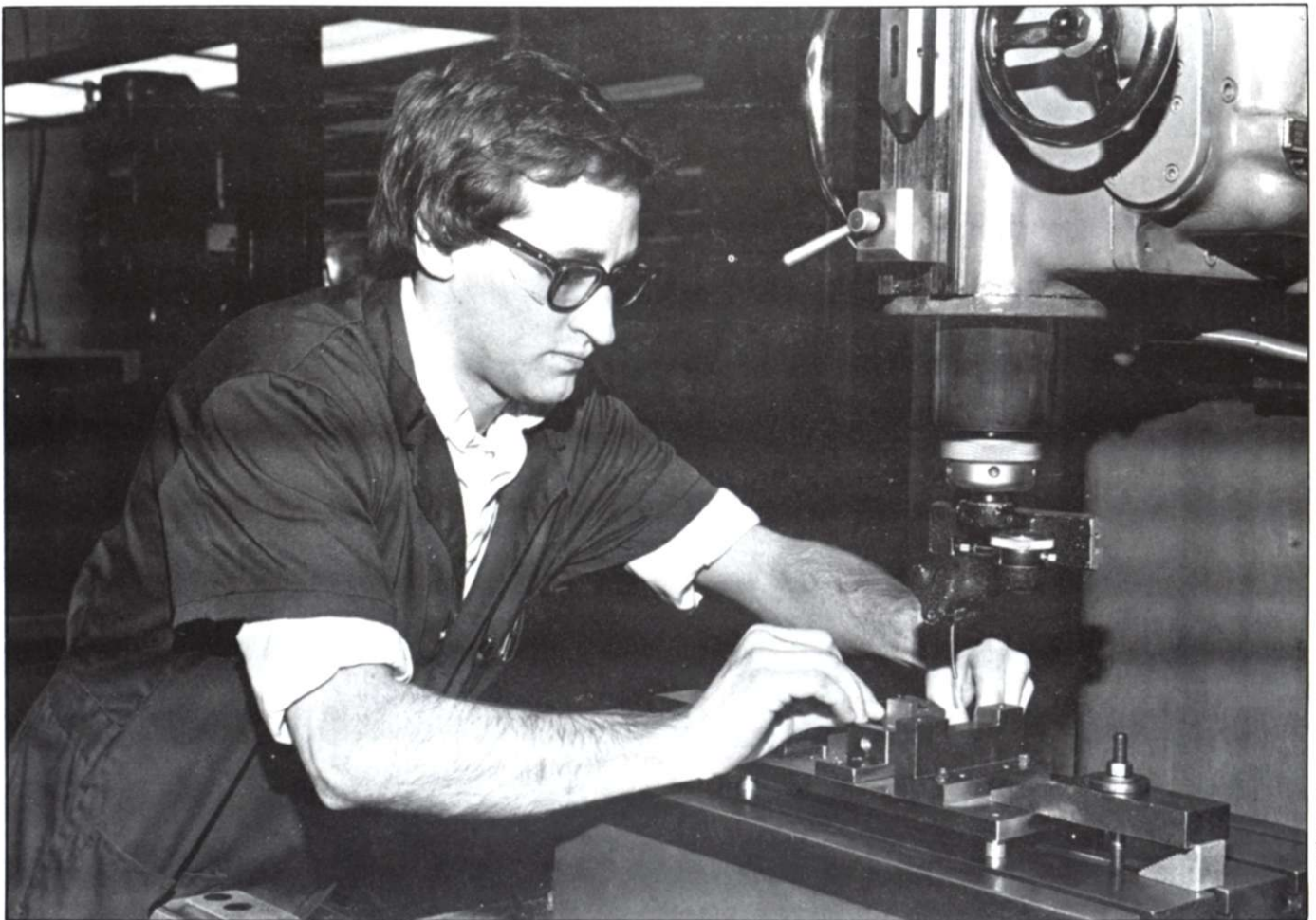
Operating the Jig bore, Roger Johnston works on one of his many projects at the RIT city center machine shop.
