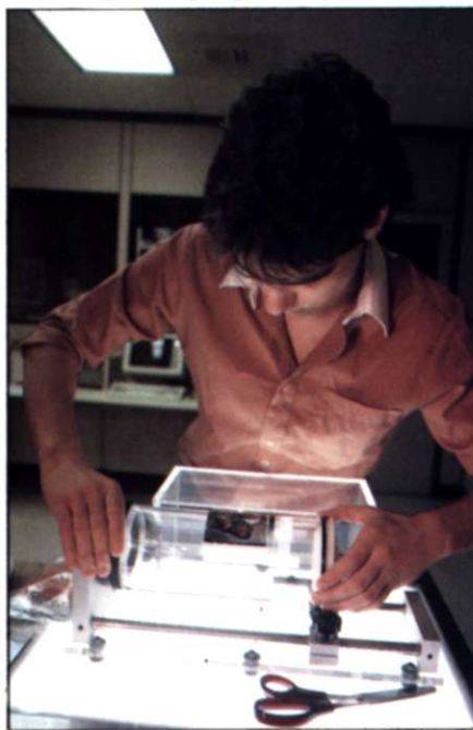
Alan R. English/T&E Center Student mounts transparency onto input scanning cylinder.
