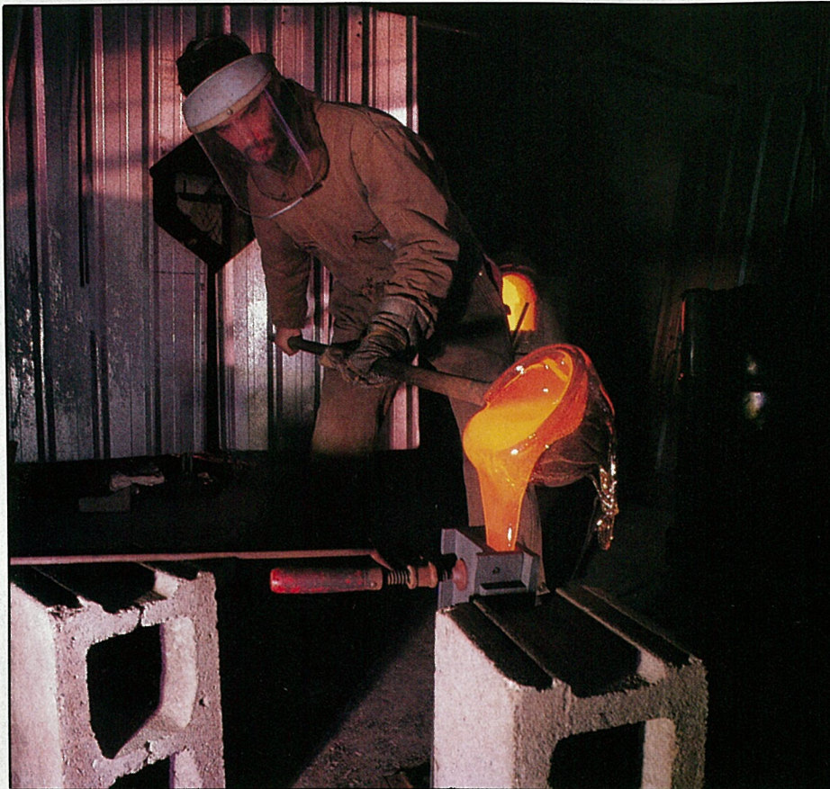
Joe O'Brien, a third year graduate student working on his thesis, prepares his cast by pouring glass into a graphite mold.
