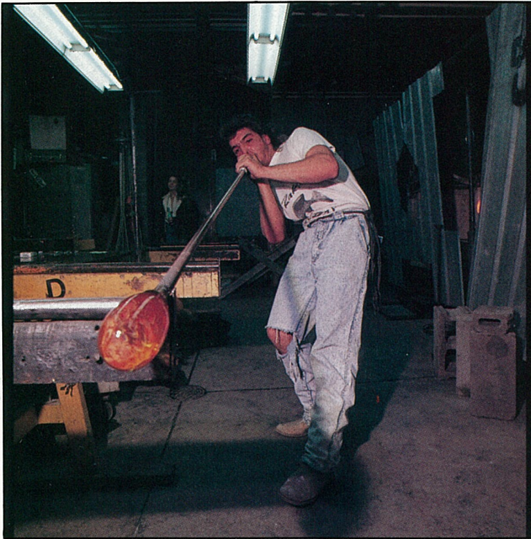
To get the shape of the glass, Jason blows into one end of the pipe.
