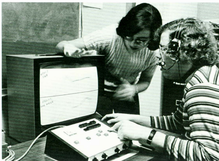
SEEING SPEECH —Speech pathologist Charissa Rubinstein explains the Visual Speech Training Aid (VSTA) to a student. The new device shows a student's speech characteristics.
