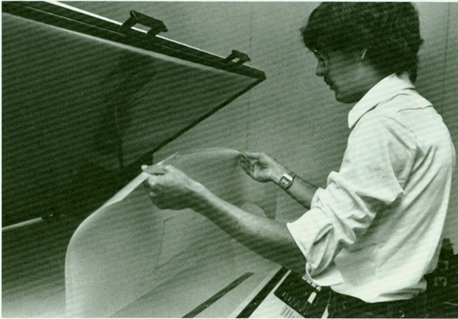
(Below) Scarpelli prepares a blueprint at his drafting table and (left) makes a copy of it on a vacuum frame device.
