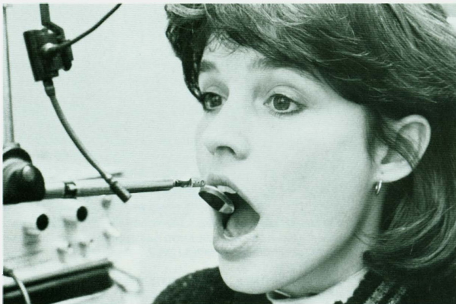
High speed cinematography Top and above, Dr. Robert Whitehead, chairperson of NTID's Communication Research Department, uses powerful lamps and heat filtering mirrors to photograph the motions of the larynx.
