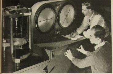
A Tensile Test Of A Steel Bar As A Laboratory Project In The Mechanical Department
