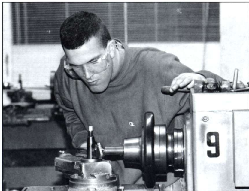
School SAE, president Moses Provenzano uses a lathe in the mechanical engineering fabrication lab to machine a part for their formula car.
