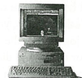
Power Macintosh 7200/75 w/CD 8MB RAM/500MB hard drive, PowerPC 601 processor, quad-speed CD-ROM drive, 15" color monitor, keyboard and mouse.
