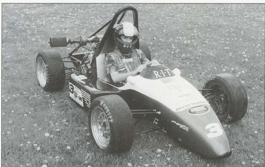
OUTSTANDING IN ITS FIELD... RIT heads to its sixth Formula SAE competition May 27-31 in Pontiac, Mich. This year's car features an 8-pound fiberglass body (compared to 26 pounds last year), a completely redesigned pull-rod suspension and enhancements to the brakes. RIT, which has taken a third- and two second-place finishes in the past four years, will compete against 110 schools in the international event sponsored by the Society of Automotive Engineers. Here, project manager Dan Tiley sits behind the wheel.
