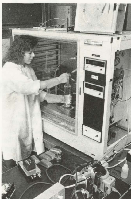
Cathy Erbland, assistant scientist at IPI, adjusts the humidity control apparatus for IPI's prototype testing chamber. The chamber will be used to explore the effects of air pollution on microfilm.
