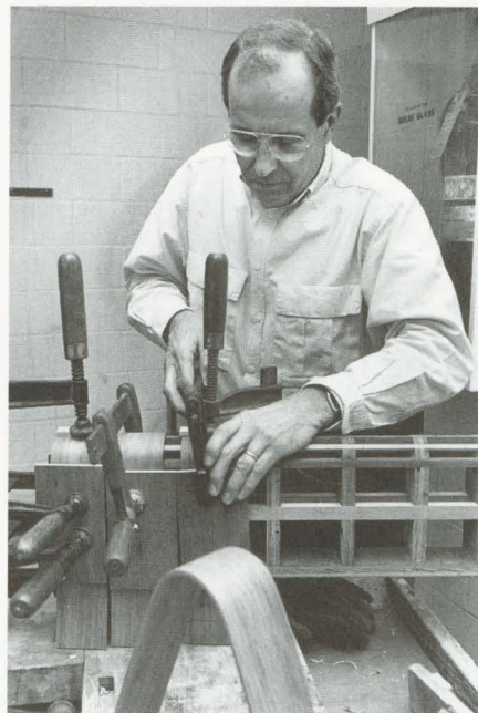
Woodworking professor Bill Keyser created a gift for Jimmy Carter in honor of his May 1 visit to RIT. The curved-corner box made of rosewood and pecan required steam-bent pieces to produce a “semi-organic” look.
