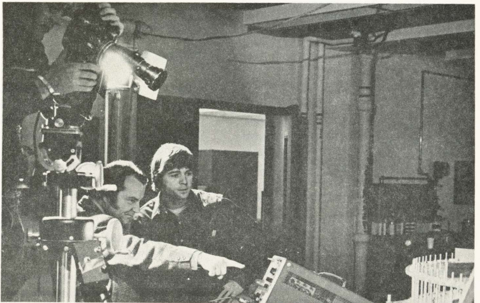
High speed filming of the flow of fluid through this water table will enable Dr. Neville Rieger (center) to measure the forces that cause failures in turbomachinery. The $20,000 water table was constructed by Alfie Wicks (right), a research associate in mechanical engineering at RIT. The filming is being done by Larry McKnight (upper left), a photographer in the RIT Media Design Center.
