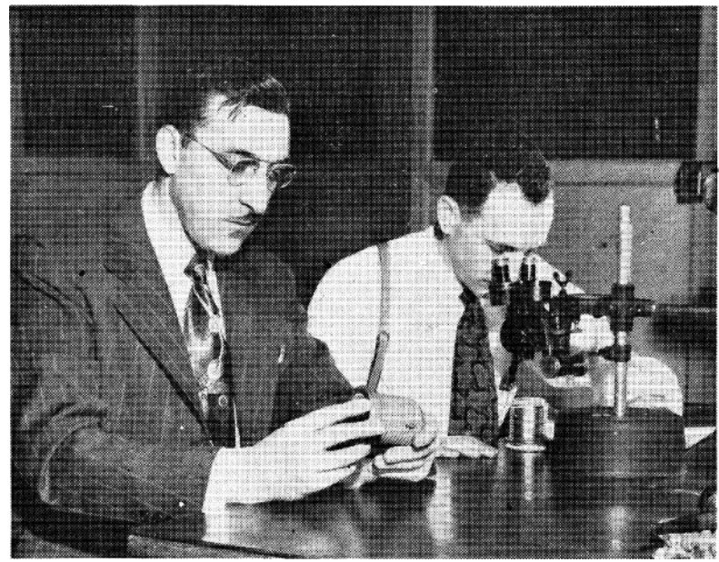
A piece of metal specimen is examined by Mr. Finsterwalder. The specimen will be checked by one of his associates under a special high-power microscope. These parts were rejected because they did not meet the rigid standards of Taylor Instrument Companies and will undergo testing in this department to find the reason for the flaws.
