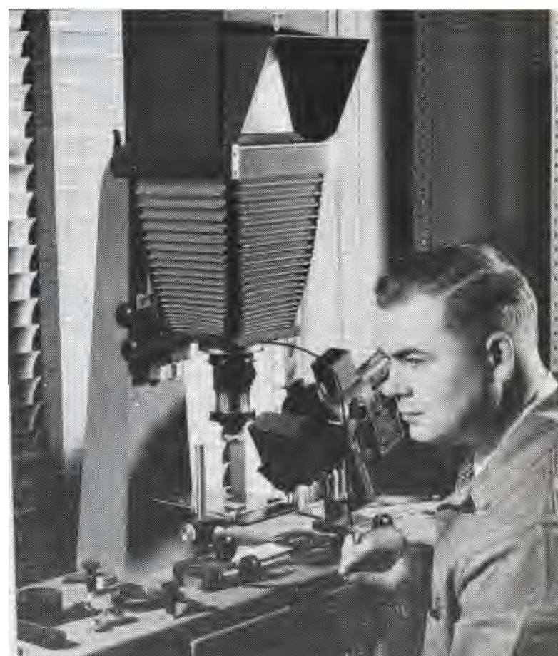
Virgil P. Barta, physicist and technical supervisor of the Research Division, is shown at the photomicrographic equipment set-up in the physics lab, applied science section. Enlarged portions of printed reproductions are photographed and studied to evaluate quality and determine physical structure of materials. Cross-sections of paper may be enlarged many times and photographed to show fiber patterns and surface coating.
