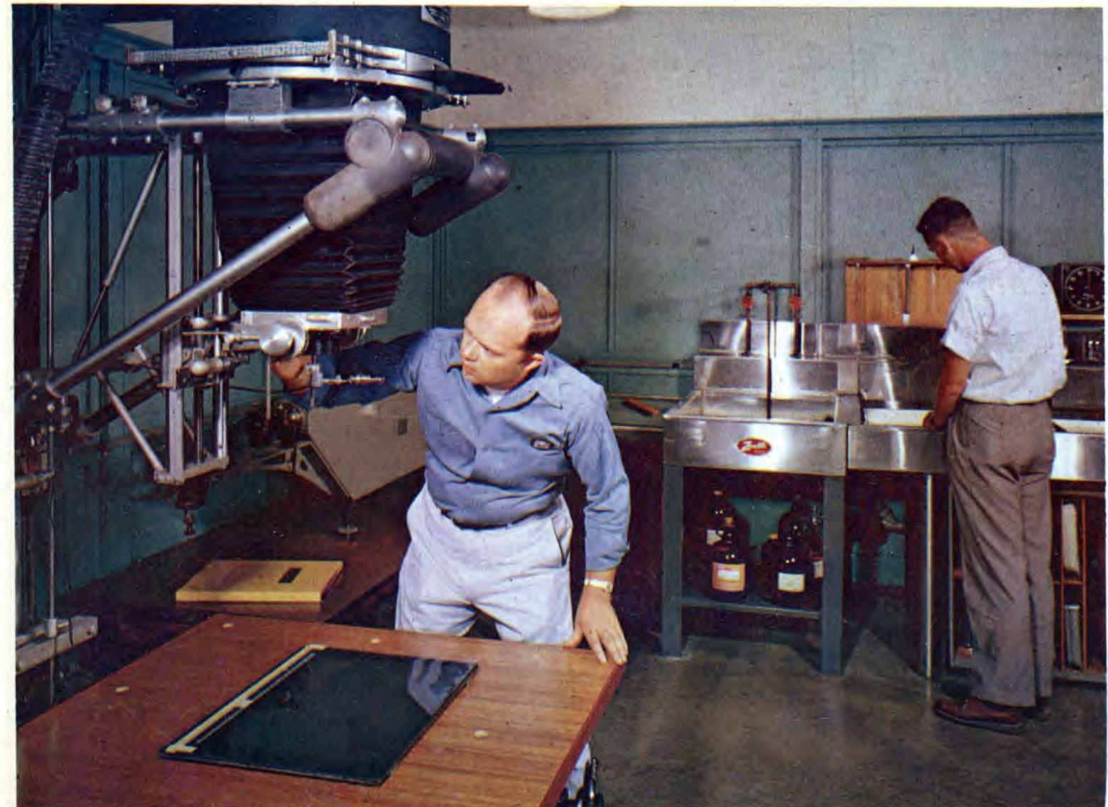
COLOR SEPARATION DARKROOM Separations are made directly from transparent originals to be used in conjunction with web offset newspaper production project. Temperature control is utilized and techniques are standardized to insure uniform color balance.
