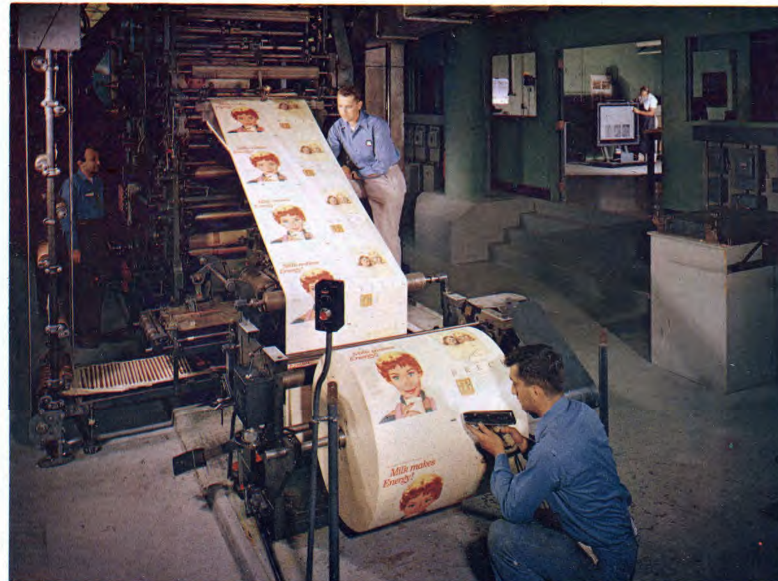
4-COLOR WEB-FED OFFSET PRESS This perfecting press is utilized as research equipment for testing paper, inks, blankets and plates. It is used to solve problems and develop new production techniques in the area of offset press operation.
