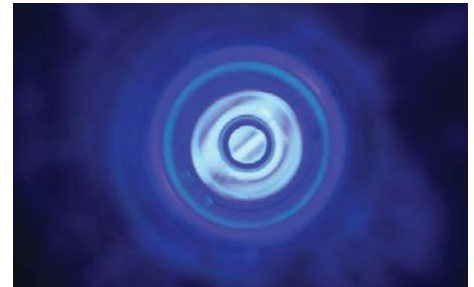
Photoluminescence from ZnS quantum dots prepared in the NPRL
