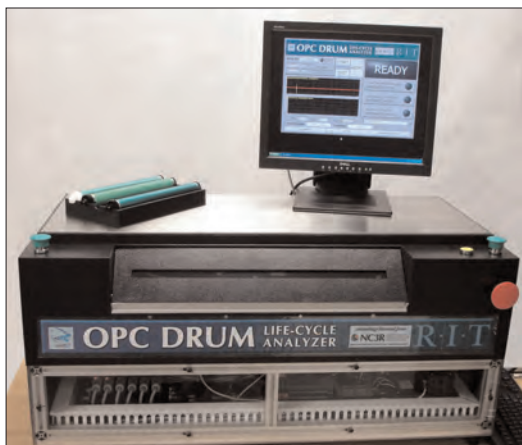
The OPC Drum Life Cycle Analyzer will drastically reduce the waste associated with remanufactured printer cartridges while also decreasing production costs and increasing efficiency.
