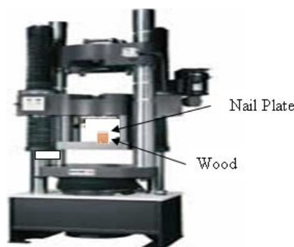
Figure 4. Compression test of the nail plate to a wood pallet
