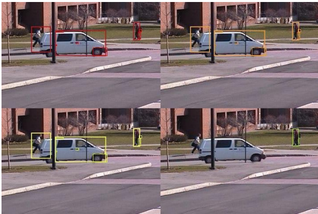
Figure 9. The IVEE subsystem habituates similar events that occur at the same time each week.
