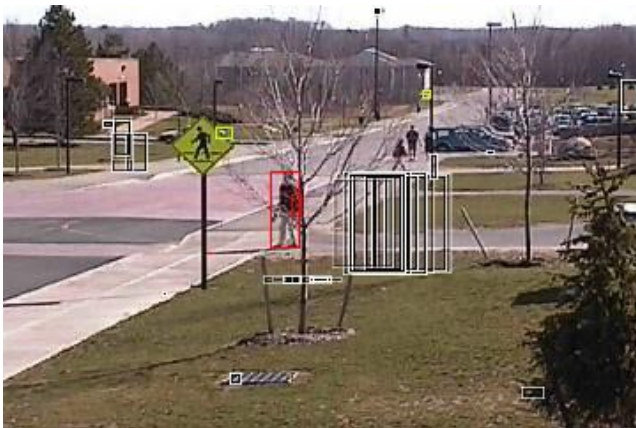
Figure 10. The IVEE subsystem draws black and white rectangles, which indicate where missed expected events have occurred.
