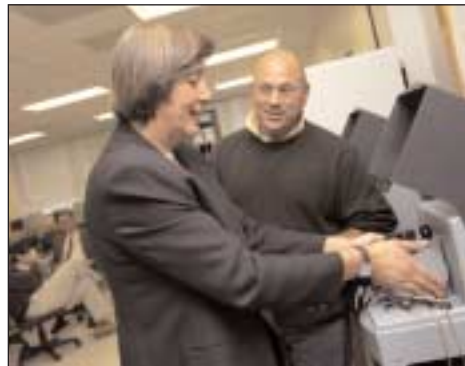
Maria Rubino and Fritz Yambrach, packaging science professors, inspect a device used to test water and vapor permeability in plastic packaging in RIT's new Integrated Plastics Center in CAST.
