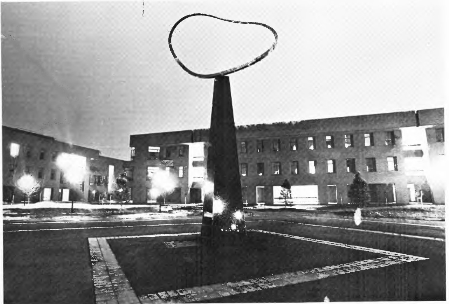
The Jose De Rivera sculpture in the science quad is powered by a \frac{1}{4} -h.p. motor to revolve once every one hour on a 12' high triangular base
