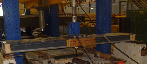
Figure 4. Test set up for bending experiments
