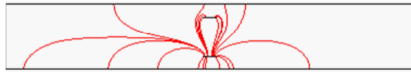
Figure 16. Streamline plot of the potential distribution of the broadside-coupled stripline with port 1 as input
