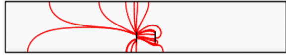
Figure 8. Streamline plot of the potential distribution of vertical plate broadside-coupled stripline with port 1 as input
