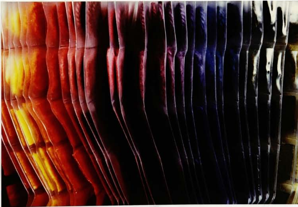
Fig. 6. Dye Notebook testing color results of benzyl dyes on wool and silk.
