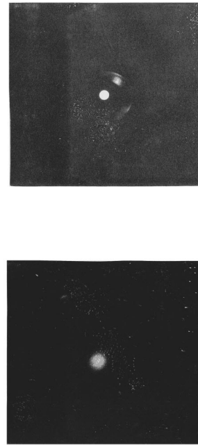
FIG. 15. Mylar witness plate: (a) Image of the electron beam after it transmits through a 0.051 mm Tantalum foil, (b) image of the electron beam after it passes through a 0.10 mm Tantalum foil.
