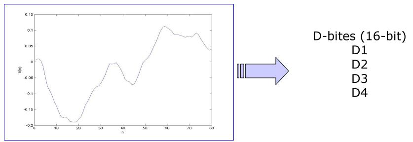
80 points of a sound wave replaced with 4 critical points, resulting in a 20:1 compression ratio
